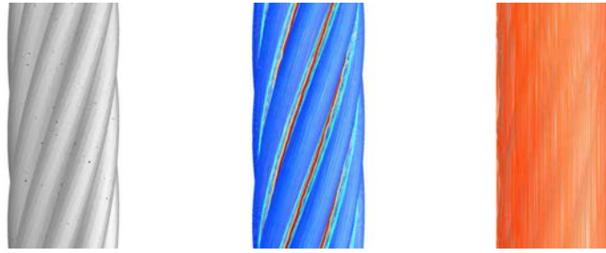
Figure 3.5: Minimal curvature lines. Left: input shape (already introduced in Figure 2). Middle: a low scale produces lines following the small twisted cables. Right: at high scale, the minimal curvature lines follow a vertical straight cylinder. Colors are based on |\kappa_1| - |\kappa_2| from 0 in blue to 3 in red.
