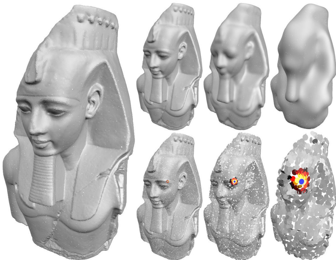
Figure 1.9: Multi-scale and multi-resolution representation. Top right: three results of the projections of 1M initial points (left) at scale levels 10, 20 and 30 among 50. Bottom right: the corresponding sub-sampled point clouds with \alpha = 0.1 (Equation 1.41). The heat map highlights the neighborhood used to compute the APSS for the same blue point at the three scales.
