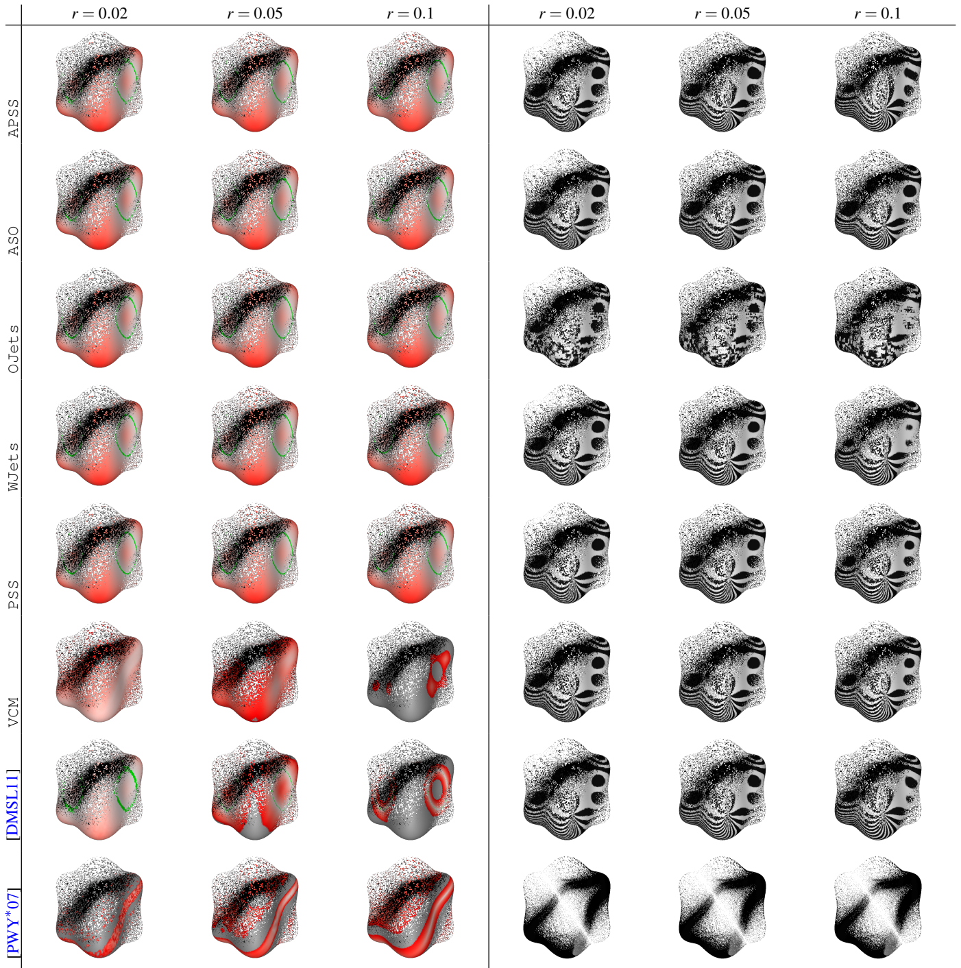
Figure 9: Mean curvature and normal vector estimations on an highly non-uniform sampling of the Goursat's surface.
